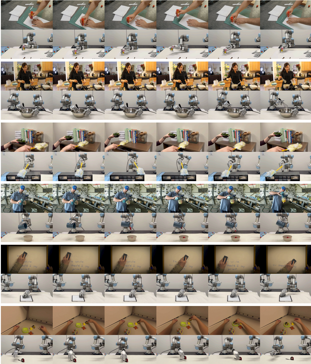
Figure 12: Real-World Rollouts. Frames from our robot rollouts for spreading, whisking, dusting, pouring, erasing, and picking. More tasks and videos are available on our webpage.
