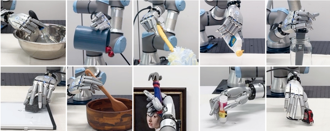
Figure 6: Real-World Deployment. We showcase trajectories for 10 tasks: whisking, pouring, dusting, squeezing, tamping, erasing, stirring, hammering, spreading, and picking.
